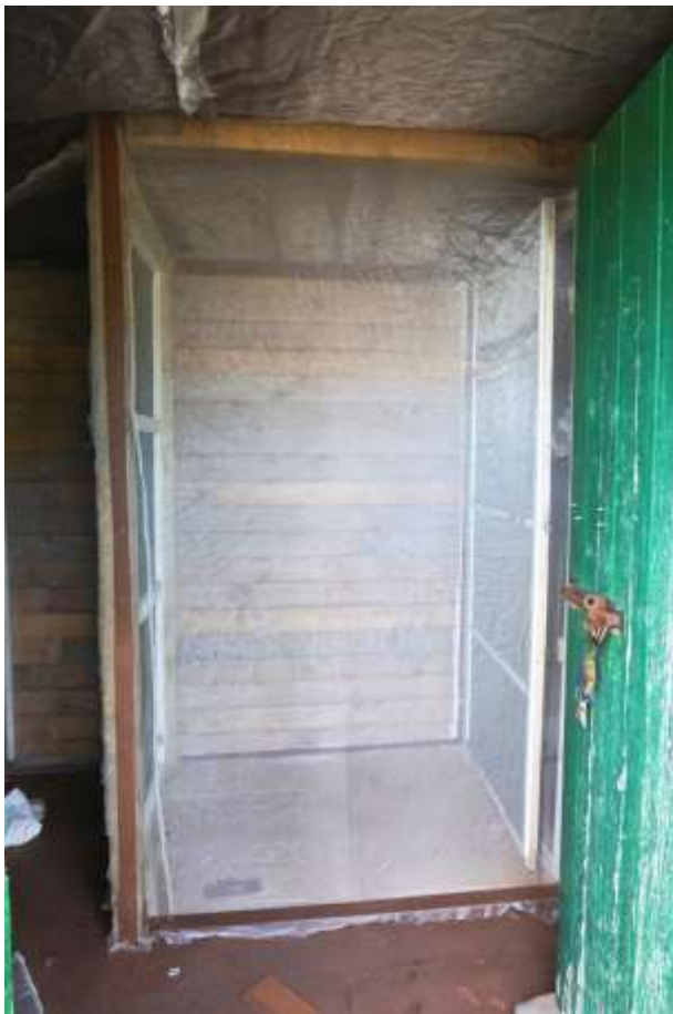
Figure 2: Double door entry system into the inner quarantine chamber
